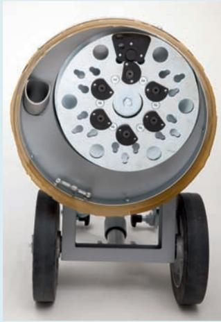
The **dust hood** has been completely redesigned. It is no longer fixed rigidly and is fitted with a double, flexible sealing ring guaranteeing dust protection.
