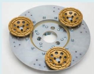
**Diamond drive plate, buffered**, Ø 400 mm, for various tools, e.g. 3 double-rowed diamond cup wheels, Ø 125mm, for keying concrete, screed, etc.
