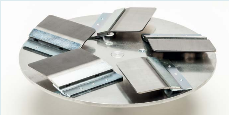
Bladed planing disk Ø 300 mm, wide-angled , with 5 steel planing trowels (20°) for smoothing the surface of finished floors (concrete, screed)
