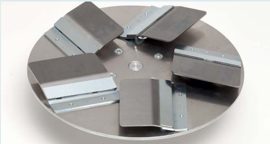
Bladed planing disk Ø 300 mm, sharp-angled , with 5 steel planing trowels (16°) for pre-planing surfaces
