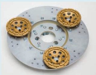
Diamond drive plate, buffered , Ø 400 mm, for various tools, e.g. with 3 double-rowed diamond cup wheels, Ø 125 mm, for keying concrete, screed, etc.
