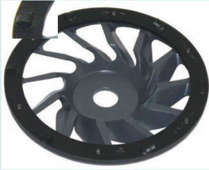
PCD cup-wheel DFT-175, BLACK, Part no. 220.400 with 6 PCD-segments, for the removal of all stubborn adhesives (PU, bitumen, synthetic resin, dispersion adhesive, tile and powder adhesive), filler, felt paper, plaster PCD ring wearing part DFR-175 BLACK, Part no. 220.410
