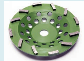
DIAMOND-cup wheel TURBO GREEN for extremely hard concrete, DT-175-TURBO-16/20 Part no. 223.241 Grain 16/20 for grinding of extremely hard materials such as screed/ concrete with floor hardeners, natural stone, stoneware DT-175-TURBO-30/40 Part no. 223.242 Grain 30/40 coarse sanding DT-175-TURBO-60/80 Part no. 223.243 Grain 60/80 medium sanding DT-175-TURBO-120/140 Part no. 223.244 Grain 120/140 fine sanding
