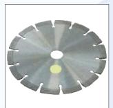
2. Diamond cutting disc `Concrete` Ø 150 mm Part no. 239.158 10 mm segment height, bore hole 22,23 mm, for concrete, reinforced concrete, aggregate concrete, common construction material
